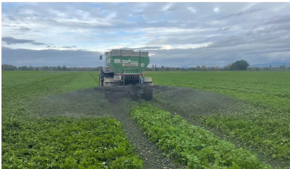
Figure 2: Rock powder application using a widely available lime spreader. (Photo: Matthias Huber of Lindenhof, Achern, Germany, 2022).
